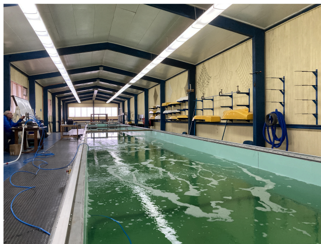
Fig. 3. Hydrodynamic testing channel.
