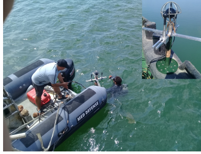
FIG. 4. Experimental setup showing diver, sensor platform (hydrophones + AVS), and support boat.
