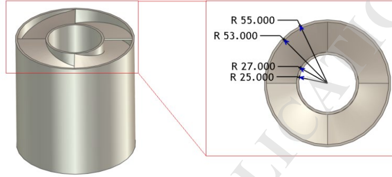
Fig. 4 The basic dimensions of the acoustic metamaterials muffling unit
