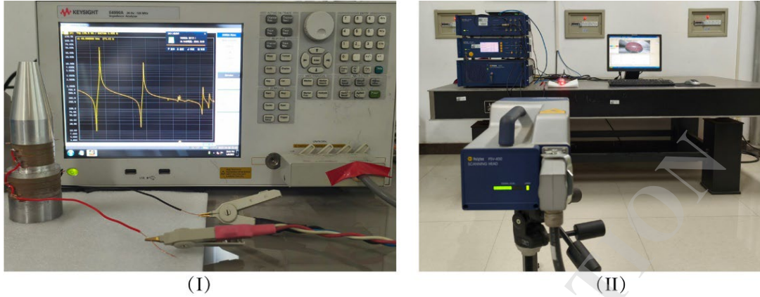
Fig. 16. (I) Measured the electrical impedance frequency response of the transducer by using the E4990A precision impedance analyzer; (II) Measured the vibration mode of the transducer by using the Polytec scanning vibrator.
