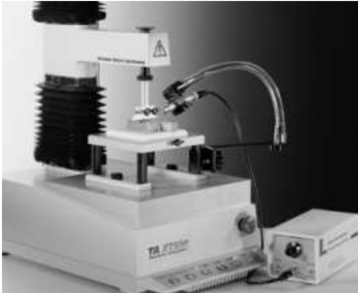
Fig. 1. The texturometer of type TA XT plus, produced by Stable Microsystems LTD, equipped with the microphone probe and the acoustic amplifier to capture the sounds generated in the mechanically loaded food sample.
