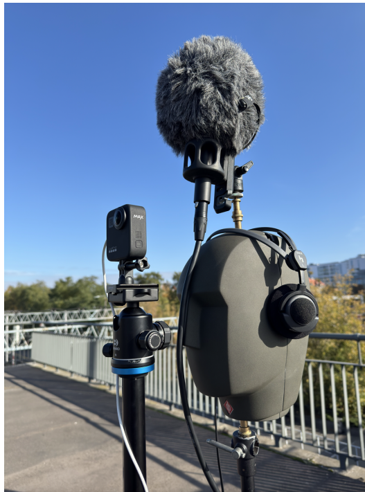
FIG. 4. Recording setup – binaural microphones, ambisonic microphone, and 360° video camera.
